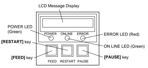
The LCD Message Display shows messages in alphanumeric characters and symbols to indicate the printer's status. Up to 16 characters can be displayed on one line.
